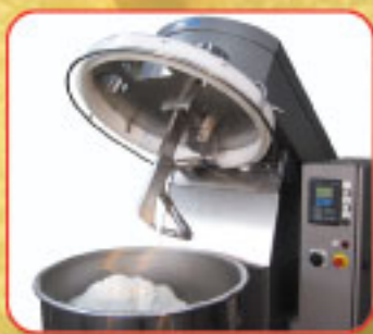
Heavy Duty Stainless Steel Spiral Agitator, Breaker Bar and Bannet Cover included
