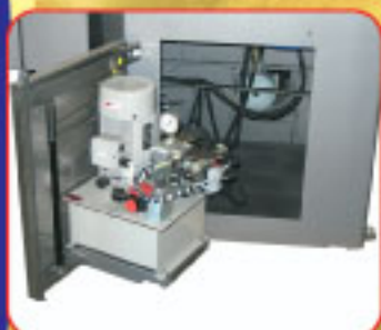
"Swing-Out" Hydraulic Package for ease of Maintenance and Sanitation
