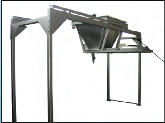
The inside of the dough hopper can be non-stick coated or made from stainless steel with a "swirl" finish for less dough sticking
