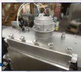
Bulk dry ingredient openings can be slide gate or butterfly style as desired.
