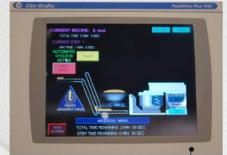
Fully graphic operator touch screen for automated control and – status indications. When used without the dough chunker-elevator, the dough can be deposited onto a mobile table or into a mobile fermentation trough as desired.
