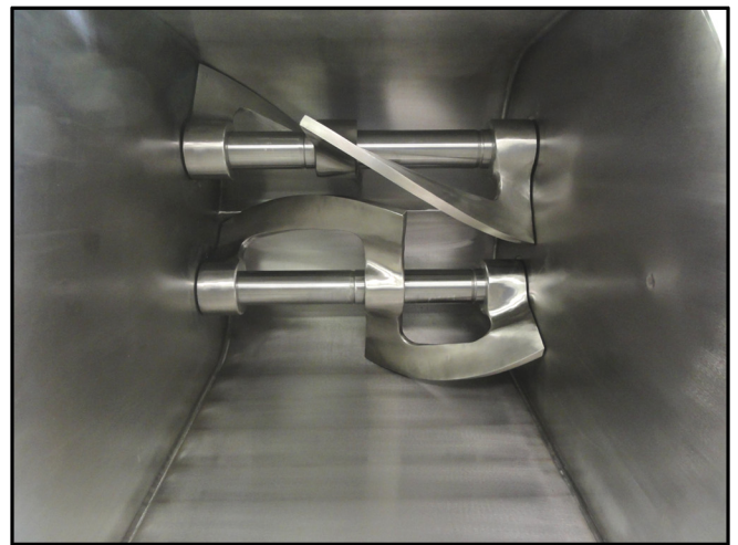
Heavy duty stainless steel agitators with overlapping design provide thorough mixing of many types of batters and doughs
