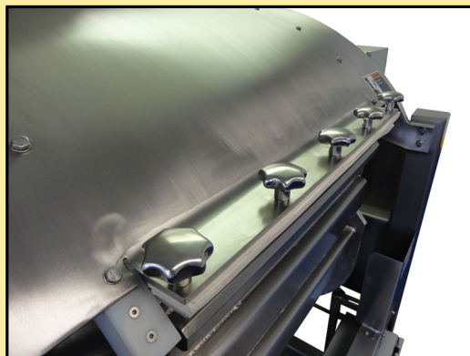
Easily removable hand knobs on both the front and the rear edge of the bowl mixing canopy allow for easy daily cleaning of these bowl sanitary seals.
