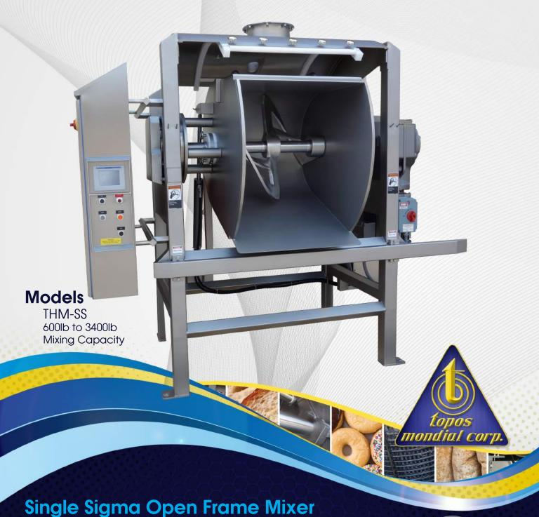
Topos Mondial can offer a Single Sigma, "Open Frame", Sanitary Designed, 110 degree overtilt horizontal mixer (SSOFHM). These mixers are being offered in several sizes [600 lb through 3000 lb]. The bowl design is a single sigma agitator design. The reinforced mixing bowl, the bowl canopy, the main shaft and the single sigma agitator are all solid stainless steel. The mixer frames can also be made using mild steel coated in "STEEL IT" or from all stainless steel.
