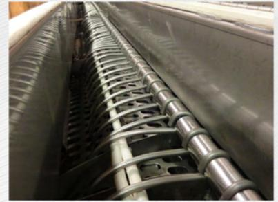
Drum fingers to reduce sugar build up on the outer surface of the inner coating drum.
