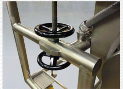
Adjustable drum angle for product flow control. Can be adjusted by hand while running.
