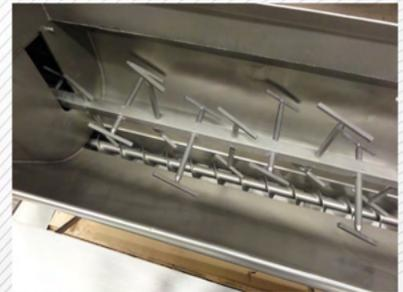
Fully agitated sugar bin with positive auger feed.
